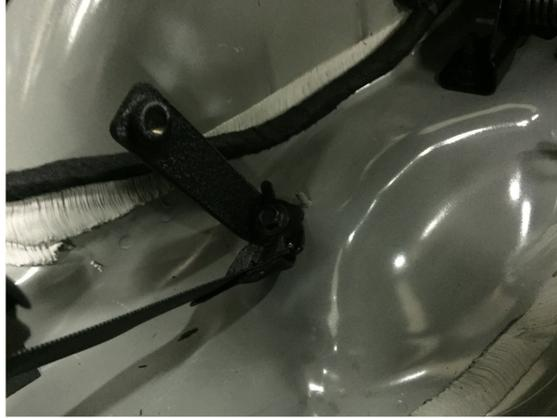
4. Temporarily install bar for alignment and spacing.
