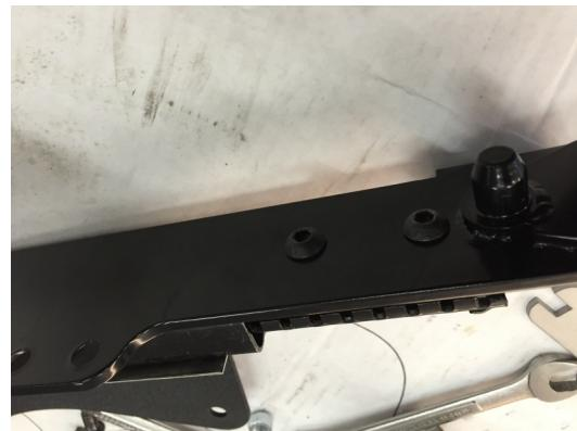
Move slider forward to allow access to lap belt mount area.
