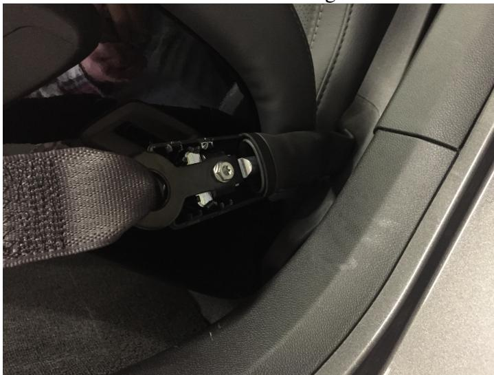
Slide the seat all the way forward and remove the rear torx bolts. Move seat to center position on slider. Lower seat to it's lowest position. Repeat on other seat. Disconnect battery ground cable at the battery. Slide the seat backwards, until the front hooks disengage, then tilt the seat forward. Disconnect seat harness, remove seat from car. Repeat on other seat if doing both seats.
