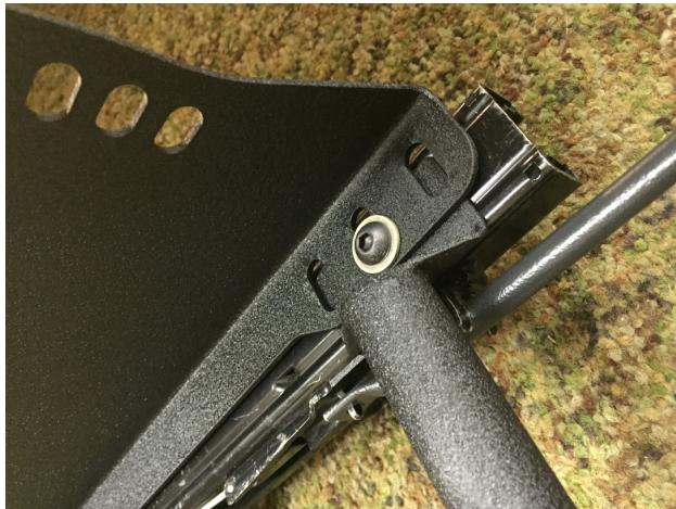
E) Side mounts. The R-9170/1 seat track adaptors are designed to work with either the R-906X line of side mounts (if using Recaro sliders) or the R-907X and R-975X line of side mounts (if bolting the side mount directly to the seat track adapter). The side mounts you use should be selected by the width of the seat you're installing in the car. Use the hardware included with the side mounts to bolt the side mount to the slider or seat track adapter.
