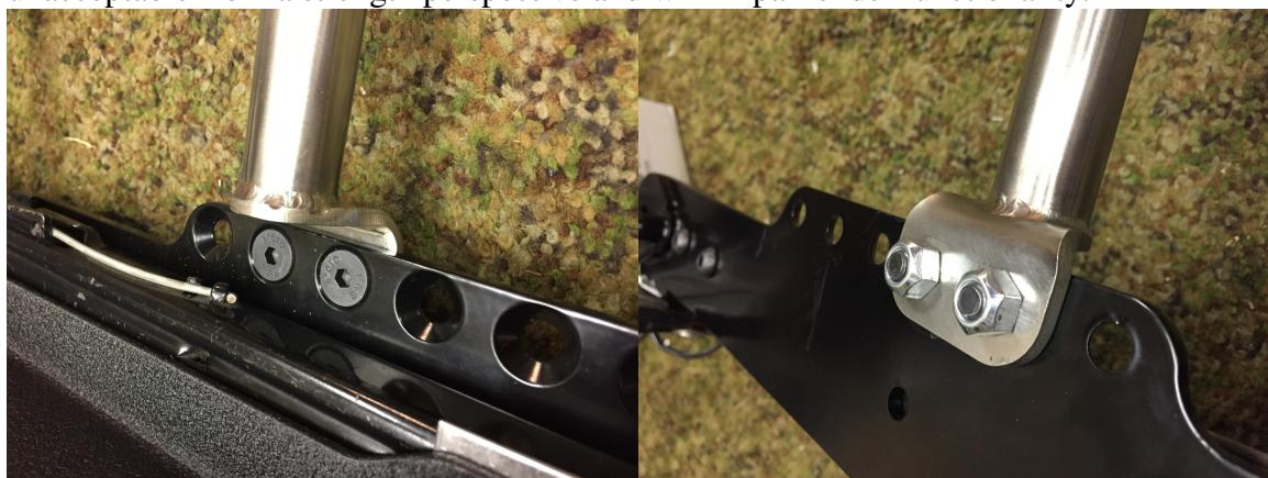
Note: Do not tighten sub strap mount to seat track adapter until seat is installed in the car, as this will set the distance between the seat track adapters (and only one distance between them will fit in the car).
